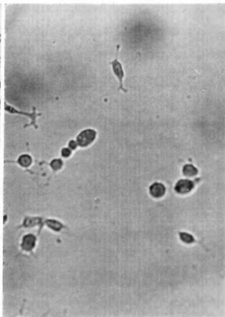
Figure 13 3T3 cell adhesion to a set of test lenses in the presence and absence of preadsorbed fibronectin . G is a HEMA based lens, whilst AD is a PEO including lens composition.
