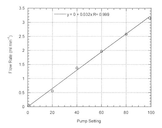
Showing Flow Rate against Pump Setting
