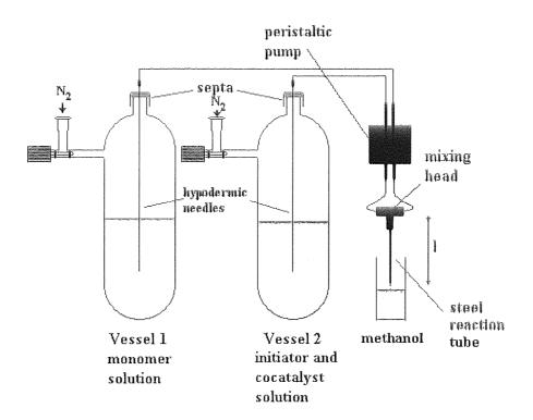
Figure 4.2. Version 1 of the Quench Flow Apparatus
