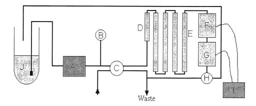
Figure 2.5 Size Exclusion Chromatography Apparatus
