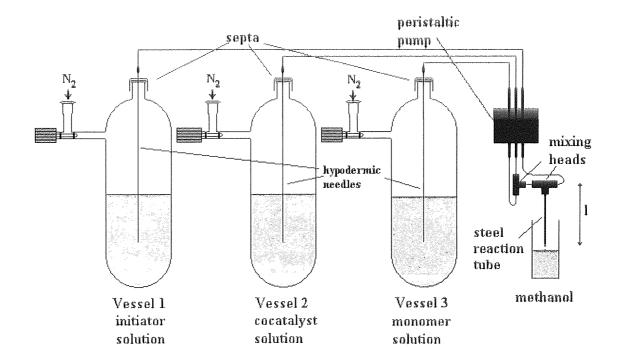
Figure 4.3 Version 2 of the Quench Flow Apparatus
