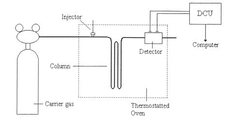
Figure 2.6 Gas Chromatography Apparatus
