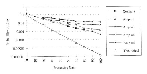
Figure 6.3 A Comparison of Different Sparse Generator Amplitudes
