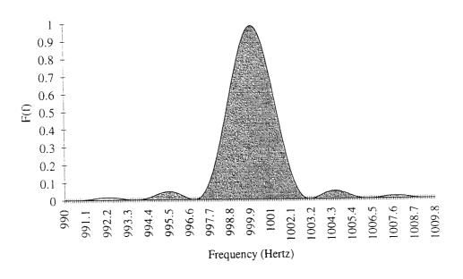
Figure 5.27 Spectrum of Spread Spectrum Signal
