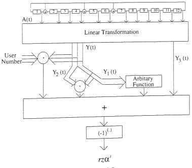
Figure 4.8 Bent Sequence Spreading Code Generator
