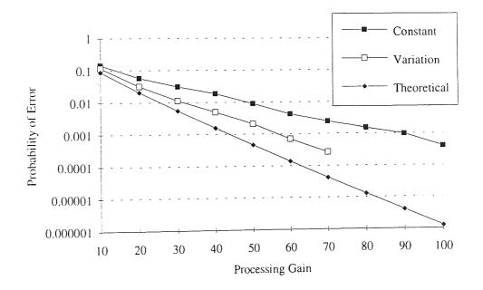
Figure 5.11 Error Probability against Processing Gain for Binary Phase Shift Keying
