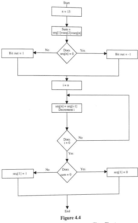
Maximal Length Data Generator Flow Chart
