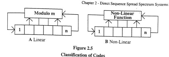
Figure 2.5 above shows schematically the two types of code generators. A, the linear generator has a feedback which takes the outputs of the registers and produces an output which is determined at that instant in modulo m logic. **B**, the non-linear generator may use past register values and any modulo calculation. In a binary system there are only two mutual operations permitted in GF(2), addition and multiplication.
