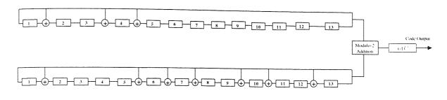
Figure 4.7 Gold Spreading Code Generator
