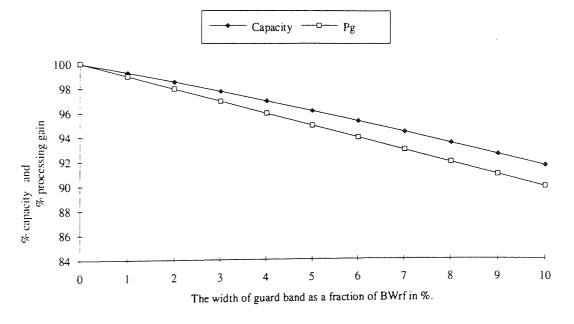
Figure 3.4 Total Capacity and Processing Gain against the Width of the Guardband
