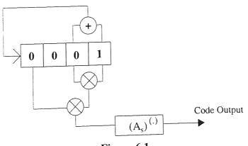
Figure 6.1 First Sparse Amplitude Code Generator
