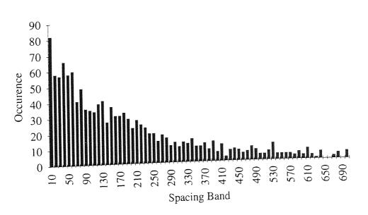
Figure 5.21 Histogram of Error Occurrence in Blocks of 10 Bits
