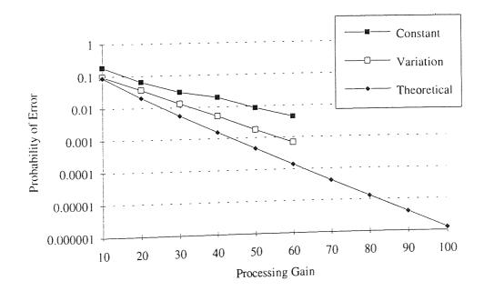
Figure 5.13 Error Probability against Processing Gain for Minimum Shift Keying
