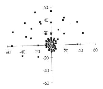
Figure 6.8 QPSK Constellation for Both Amplitude and Chip Duration Variations
