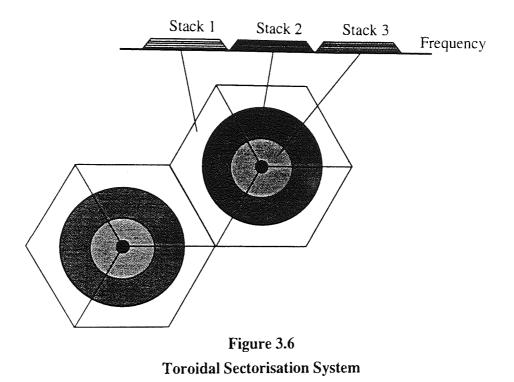
Distance ring cell splitting may be done in one of two ways, firstly by splitting the cell into disks as shown in figure 3.7a and secondly, by using toroids as shown in figure 3.7b. The disk system uses the frequency stack from the centre of the cell up to a certain radius. The toroid system uses the frequency stack between two radii.
