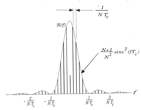
Figure 5.26 Power Spectrum of a Maximal Length Sequence
