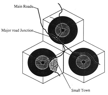
Figure 3.8 Example of Cell Clustering, Arc and Toroidal Sectorisations in Use
