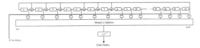
Figure 4.6 Qualcomm's Spreading Code Generator
