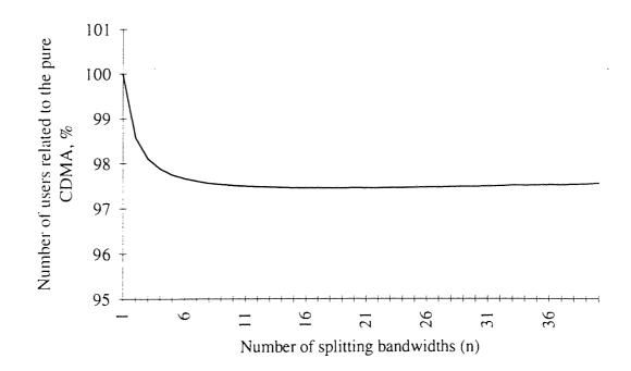
Figure 3.2 System Capacity as a Function of the Number of Splitting Bandwidths
