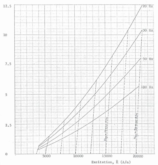
Fig. 8.2 Variation of Calculated Torque, T<sub>n</sub>, with Excitation  $\hat{K}$ , at Various Frequencies (20-100 Hz) for the End-Ring Stator.
