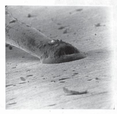
Plate 7.5 Weld, between a Nickel-Copper Wire (0.1 mm diameter) and a Steel Surface (magnified x 260)
