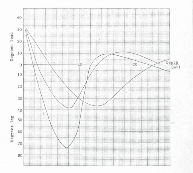
Fig. A5.2 Flux Penetration Curves: Variation, with Depth, of the Phase of the Peripheral Flux Density with respect to the Total Peripheral Flux.
