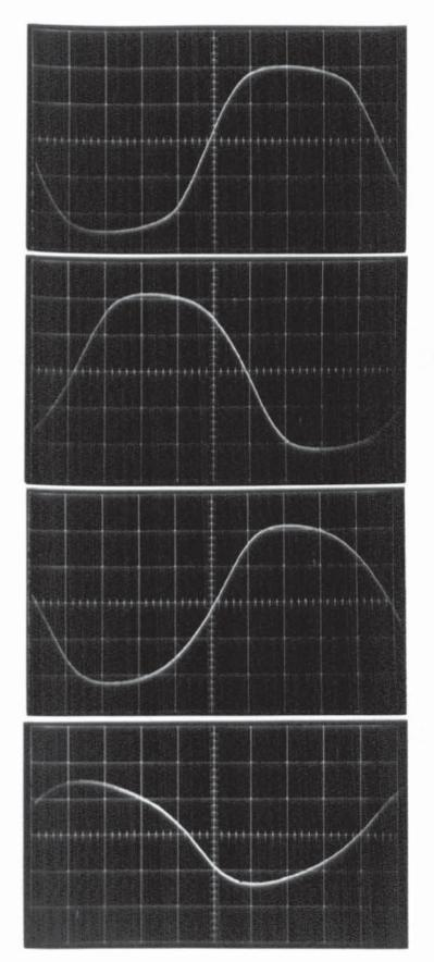
Search Coil (1) : Mean depth: 0.475 mm, Fundamental amplitude ^ 2.46 T
