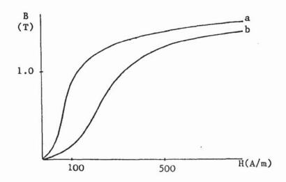
Fig. 3.3 Effect of Change in Chemical Composition on the Normal B-H curve (Bozorth <sup>17</sup>)
