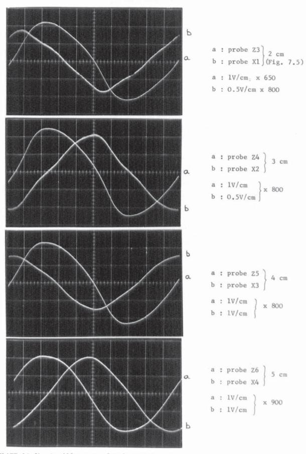
PLATE 10.2b Oscillograms of Voltages from Current Density Probes on the Continuous Stator (Fig. 7.5). Excitation: 4800 A/m; frequency:10 Hz.
