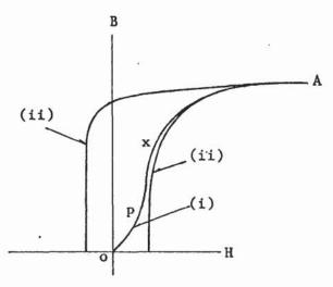
Fig. 3.1 Upper half of B-H curves for magnetic materials (Symmetrical about the H axis)
