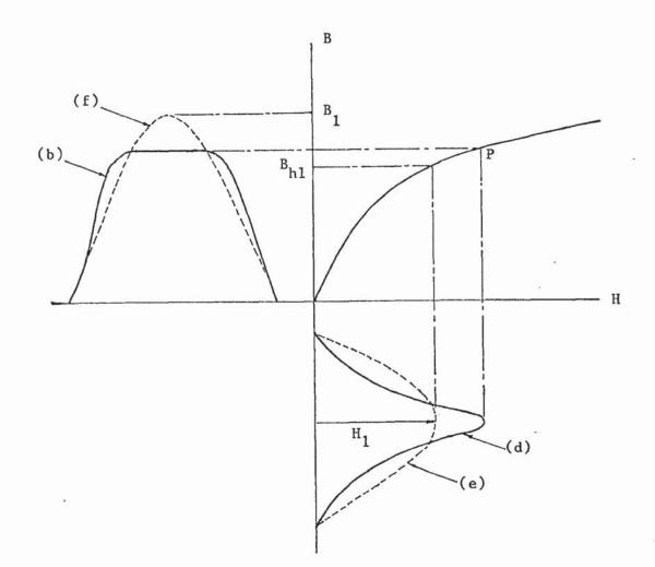
Fig. 4.4. Illustrating the Analytic Derivation of B<sub>1</sub>-H<sub>1</sub> Curves.
