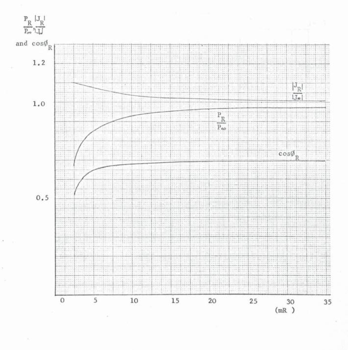
Fig. A2.2 Variation of  $\frac{P_R}{P_{\infty}}$ ,  $\frac{J_R}{J_{\infty}}$  and  $\cos \theta_R$  with  $(mR_a)$  for a Round Ferromagnetic Bar.  $m = \sqrt{\frac{\omega \mu_o \mu_r}{\rho}}$
