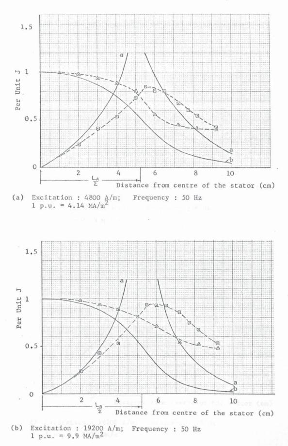
Fig. 10.9 Surface Current-Density Distribution - a Comparison of Measured and Calculated Values.
