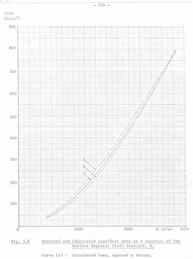
Curve (b) : Calculated loss, present non-linear theory  $(B_1 = AH_1^b)$
