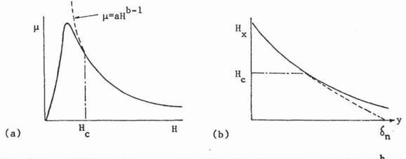
Fig. 4.1 Effect of Representing the Normal B-H Curve by  $B = aH^D$
