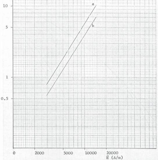
Fig. 5.7 Loss/Unit Area as a Function of the Surface Magnetic Field Strength Ĥ.
