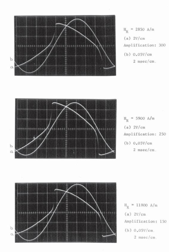
PLATE 5.1 Oscillograms of Voltages proportional to the Current Density at the Surface of the Bar (waveform (a) ), and the Current through the Bar (waveforms (b) ). (Section 5.4.2 and 5.4.3.2).
