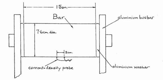
Fig. 5.4 Round Bar of EN1A Steel used in the Experimental Investigation
