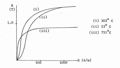
Fig. 3.4 Normal B-H curves of iron at different temperatures (Bozorth <sup>(7)</sup>)
