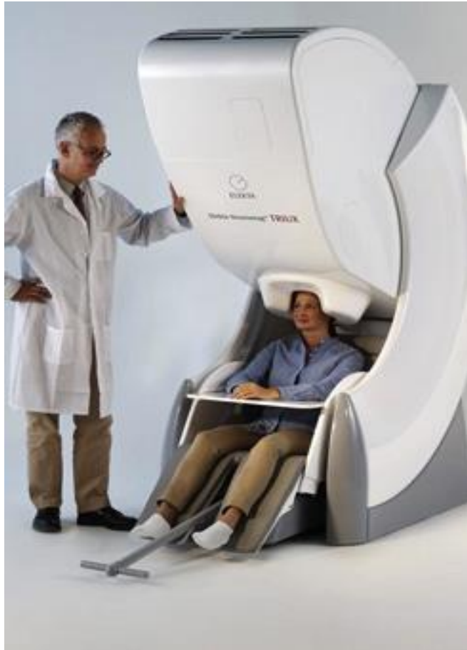
Figure 2.2 306- Channel Elekta Neuromag® TRIUX™ similar to the one available at the Aston Brain Centre, Aston University, comprising of 102 magnetometers, and 204 gradiometers.
