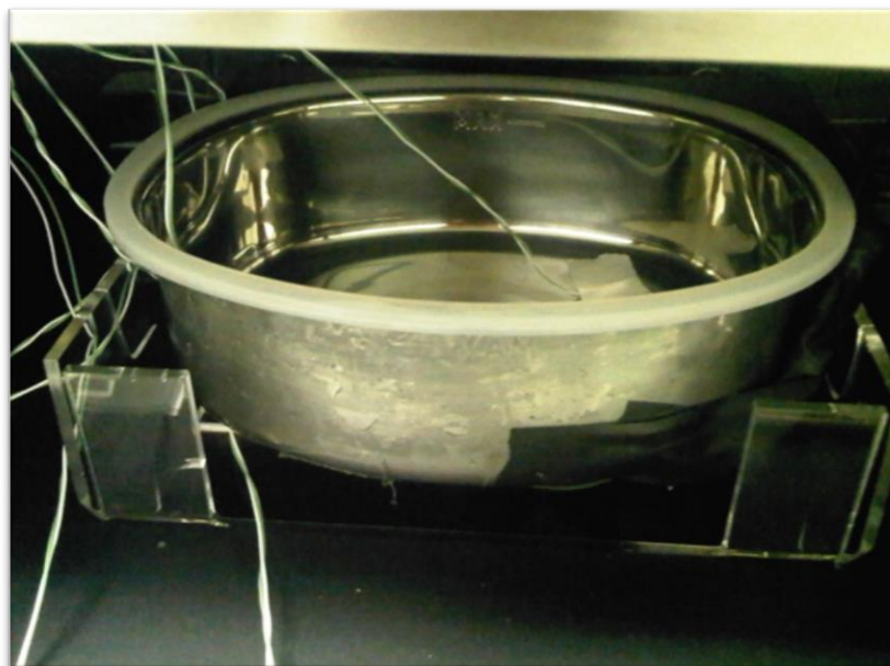
Figure 10. Straws were placed on a pre-chilled surface, inside an aluminium bowl specially built with a connection to an ultrasound transducer.
