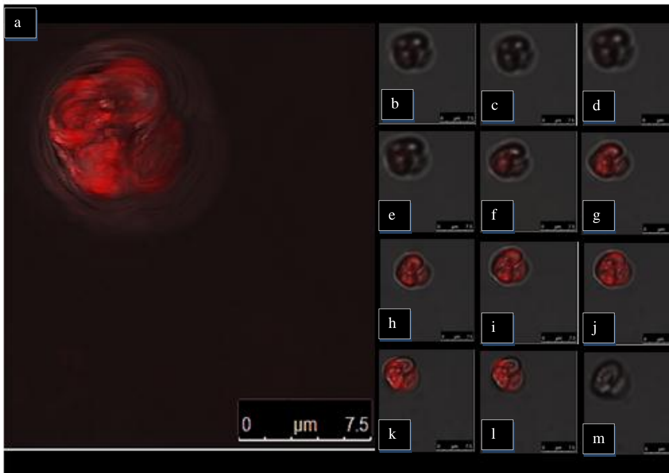
Figure 3.26 (a) The construction of a 3D visualisation of a liposome using confocal microscopy of DPPC:Chol liposomes with the fluorescent marker Dilc added at 0.2 mol %. Representative slices used for the construction of the 3D image are also shown (b – m). Aleica confocal microscope was used under a 40 X objective.
