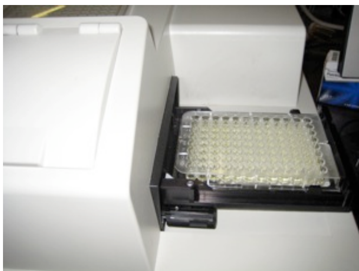
Fig 2.7. The Spectramax M2 instrument used for ELISA analysis.
