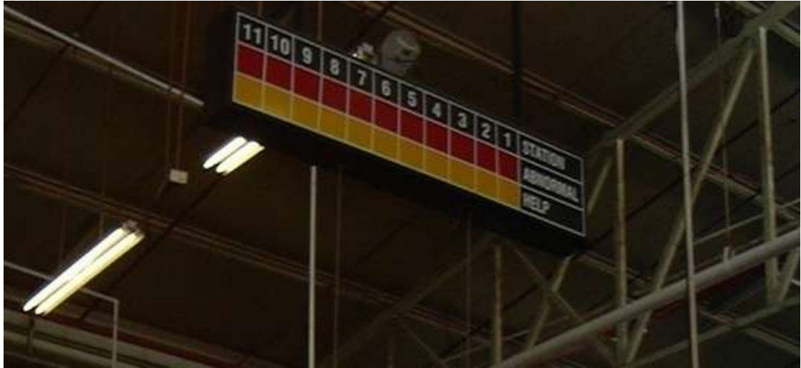
Figure 4.17: Cluster of Andon Lights at the top of production line
