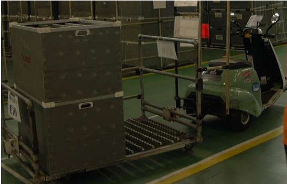
Figure 5.1: Photo of “mizusumashi” pulling trolley
