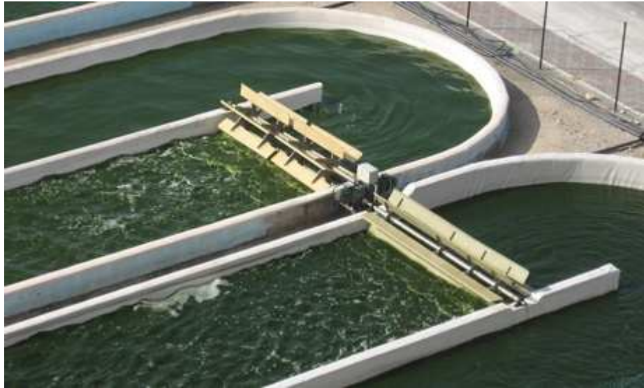
Figure 1-3 Open pond cultivation of microalgae [63]
