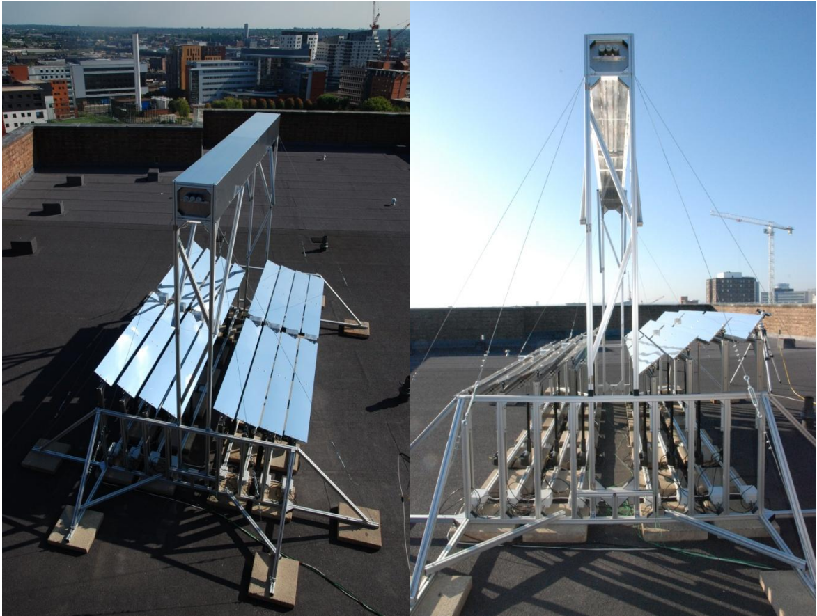
Figure 5.13: An aerial view of the ELFR (left) and the illuminated receiver during operation (right).
