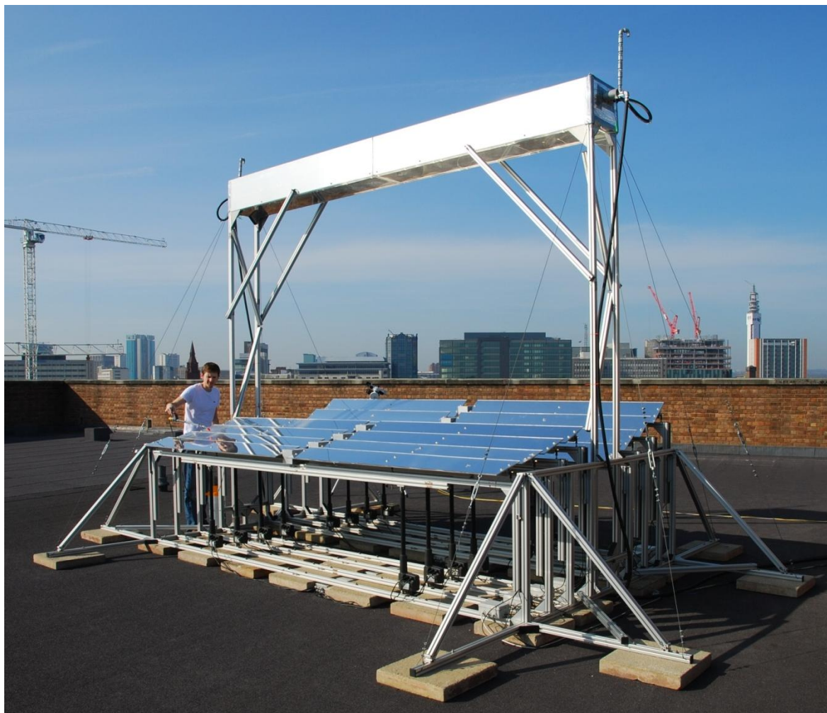
Figure 5.11: The ELFR connected to a water supply by means of a steam hose. The mirror elements were regularly cleaned using distilled water, as depicted.
