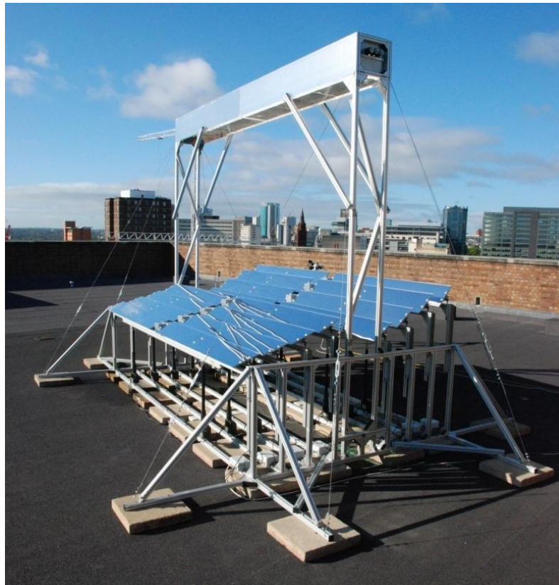
Figure 4.11: The ELFR prototype, constructed on the roof of Aston University, UK.
