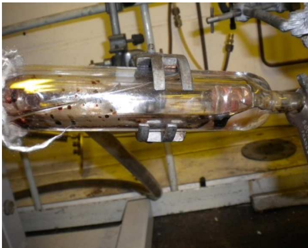
Figure 8-19: Main bio-oil condensed in water condenser / Collection of main bio-oil in pot 1
