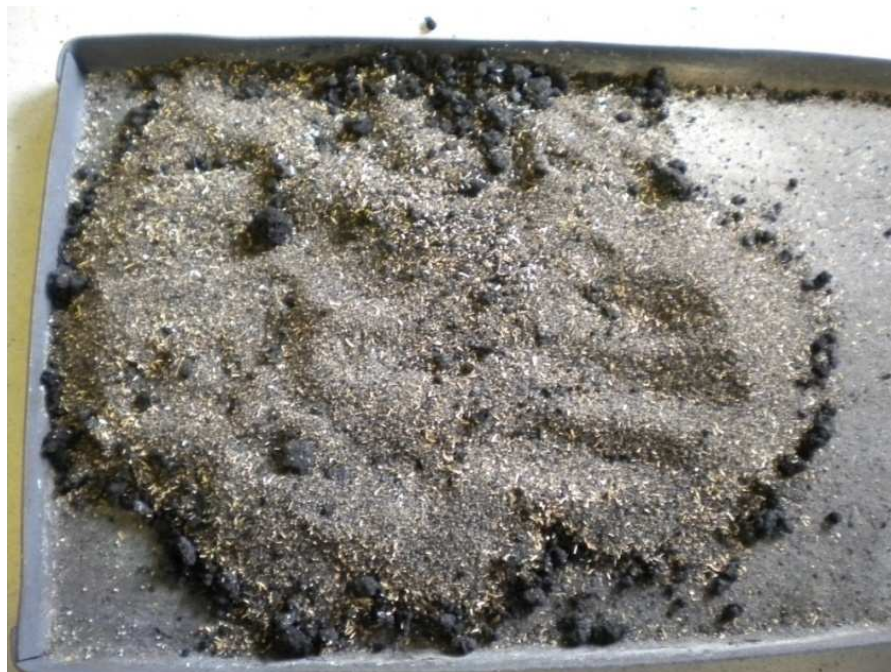
Figure 8-15: Agglomeration in fluidised bed
