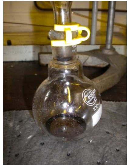
Figure 8-19: Main bio-oil condensed in water condenser / Collection of main bio-oil in pot 1
