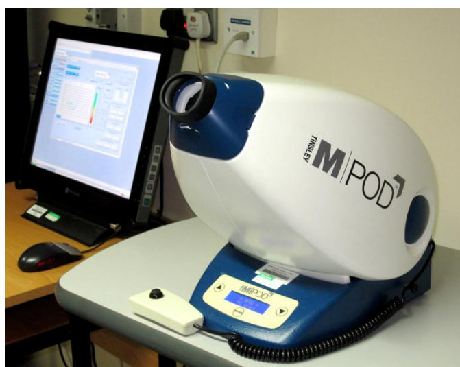
Figure 2.1 The MPS 9000 (also known as M|POD or QuantifEYE), shown with a linked computer that reveals the resulting MPOD output.
