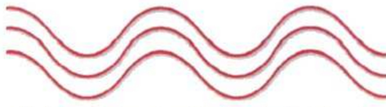
Figure 47. The light from a laser represented as waves, all in phase with each other.
