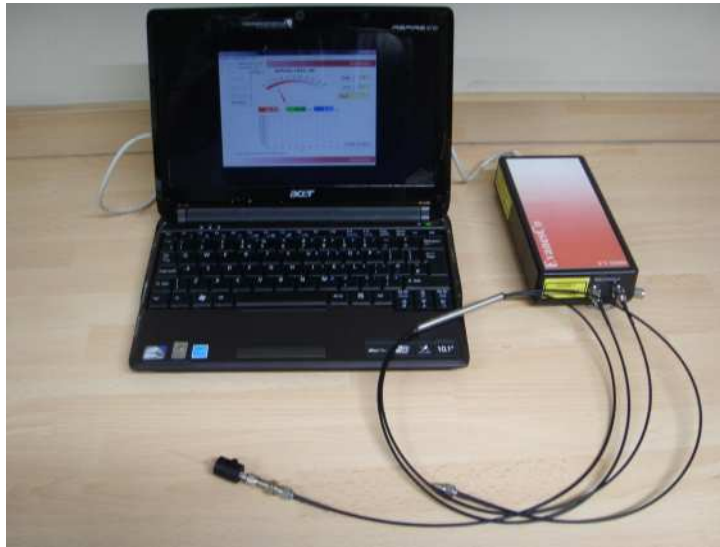
Figure 27. The EV5000 interrogation unit connected to a laptop with an end stop probe connected via a splitter/coupler.
