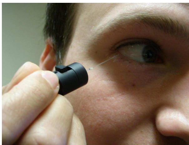
Figure 52. A straight fibre optic probe coated with a smart hydrogel being used to perform a direct assay of the lower tear meniscus.
