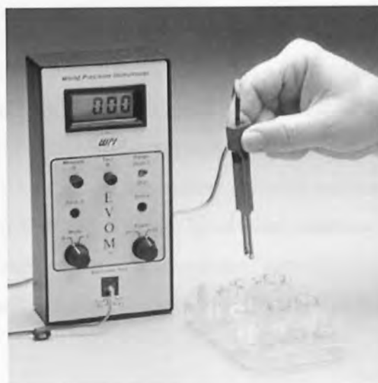
Figure 7.3 An image of the EVOM - Epithelial Voltohmmeter, showing the chopstick electrode comprised of a fixed pair of double electrodes and the EVOM resistance reader (adapted from Anon A, 2008).
