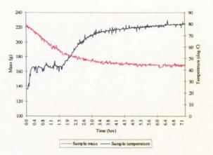
Figure B.26 Air drying of electro-porcelain  $(T_a = 80 \text{ °C}, 10 \text{ \% rh})$
