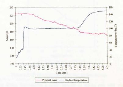
Figure 6.27 Airless drying profile: temperature and product mass (T<sub>shs</sub> = 150 °C)
