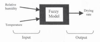
Figure 6.2 Block representation of fuzzy drying model for convective air drying and heat pump drying
