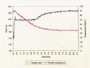
Figure B.34 Air drying of electro-porcelain  $(T_a = 90 \text{ °C}, 40 \text{ \% rh})$
