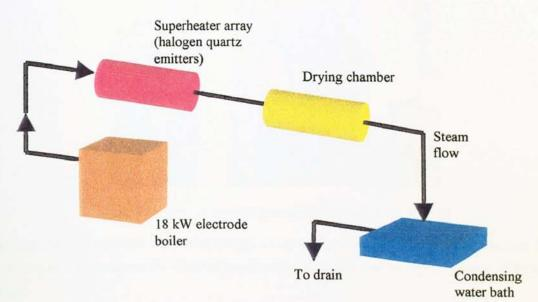
Figure 6.22 Experimental airless dryer
