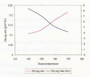
Figure 6.29 Drying time and drying rate (airless drying)
