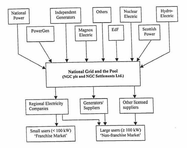
Figure 2.0 Structure of the electricity industry in England and Wales (1998) [192]
