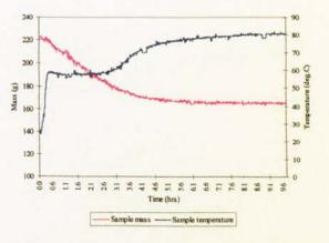
Figure B.28 Air drying of electro-porcelain  $(T_a = 80 \text{ °C}, 30 \text{ \% rh})$
