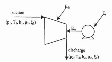
Figure 7.6 Compressor energy analysis [208]
