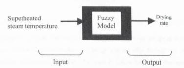
Figure 6.3 Block representation of fuzzy drying model for airless drying
