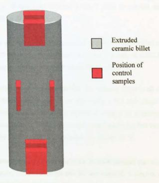
Figure 6.4 Segmentation of ceramic billet for controlled determination of moisture content
