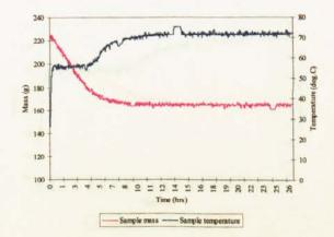
Figure B.24 Air drying of electro-porcelain  $(T_a = 70 \text{ °C}, 40 \text{ \% rh})$
