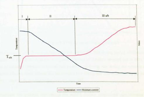
Figure 5.0 Evaporation rate curve
