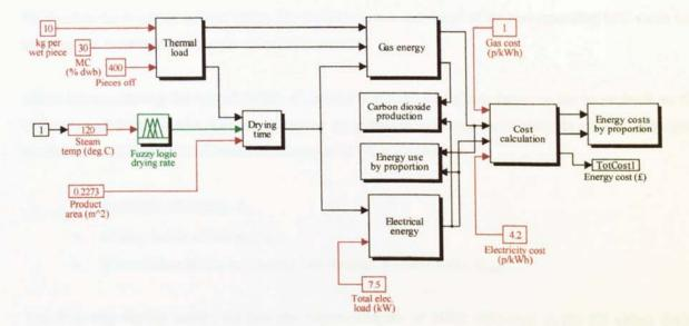
Figure 7.5 Simulink model (airless drying)
