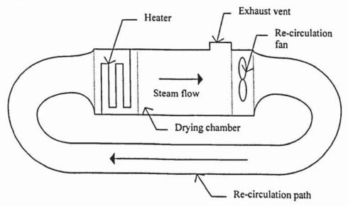
Figure 3.0 Hausbrand's concept steam atmosphere dryer [55]
