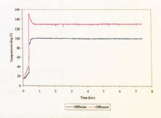
Figure B.38 Airless drying: boiler and off-heater temperature profiles (T<sub>ss</sub> = 130 °C)
