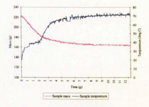
Figure B.21 Air drying of electro-porcelain  $(T_a = 70 \text{ °C}, 10 \text{ \% rh})$
