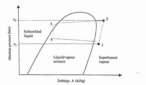
Figure 7.9 P-h diagram (heat pump refrigerant)
