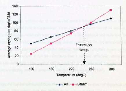
Figure 3.3 Inversion temperature for air and superheated steam drying
