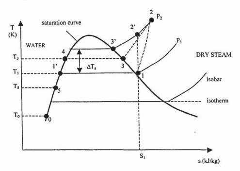
Figure 3.5 T - s diagram (mechanical vapour recompression)
