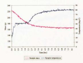
Figure B.27 Air drying of electro-porcelain  $(T_a = 80 \text{ °C}, 20 \text{ \% rh})$
