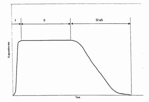
Figure 5.1 Drying curve (evaporation rate)
