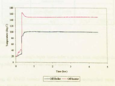
Figure 6.28 Airless drying profile: off-boiler and off- heater temperatures ( $T_{shs} = 150 \text{ °C}$ )
