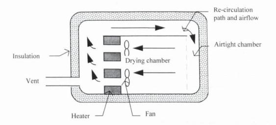
Figure 3.2 Simple outline of an airless dryer
