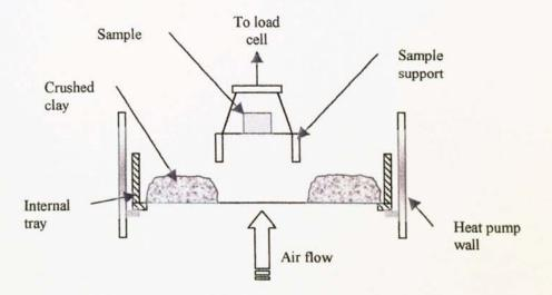
Figure 6.41 Cross section of heat pump dryer rig
