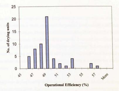
Figure 8.7 Operational efficiency for sanitaryware chamber drying
