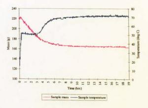
Figure B.23 Air drying of electro-porcelain  $(T_a = 70 \text{ °C}, 30 \text{ \% rh})$
