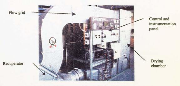
Figure 6.39 Heat pump dehumidification dryer (front)
