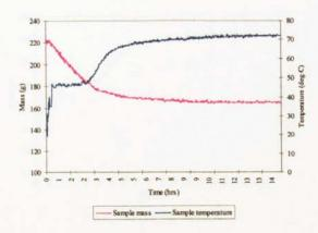
Figure B.22 Air drying of electro-porcelain  $(T_a = 70 \text{ °C}, 20 \text{ \% rh})$
