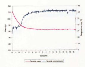
Figure B.15 Air drying of electro-porcelain  $(T_a = 60 \text{ °C}, \text{ no humidity control})$
