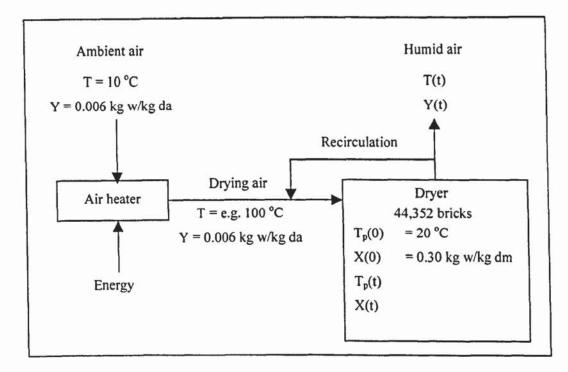
Figure 8.4 Schematic representation of an industrial dryer (after [34])
