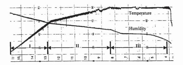
Figure 8.3 Typical sanitaryware drying profile (chamber drying)
