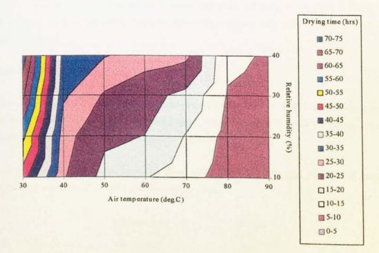
Figure 6.12 Map of drying times (convective air drying)
