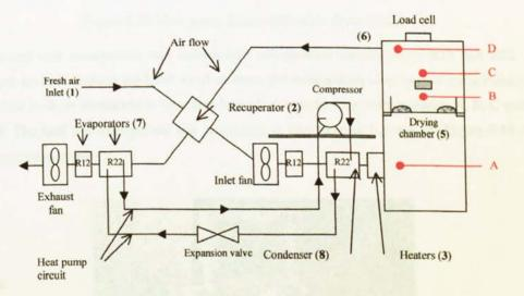
Figure 6.38 Schematic of heat pump dehumidification dryer
