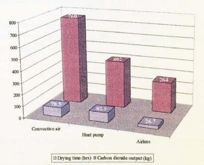
Figure 9.1 Drying time and CO<sub>2</sub> emissions
