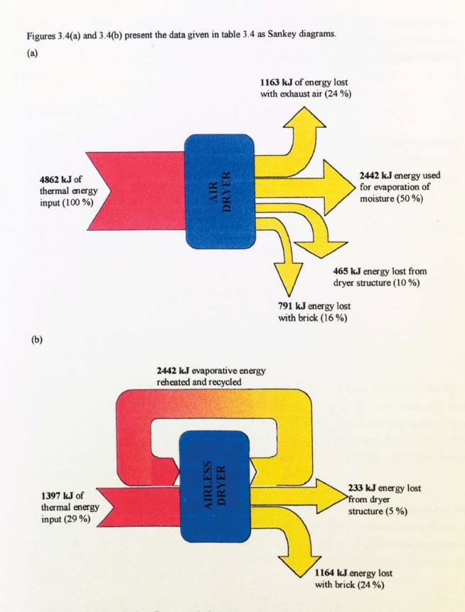
Figure 3.4 Sankey diagrams: air drying (a) and superheated steam drying (b) of brick
