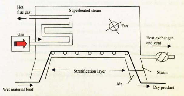
Figure 3.1 Simplified schematic of a continuous airless dryer
