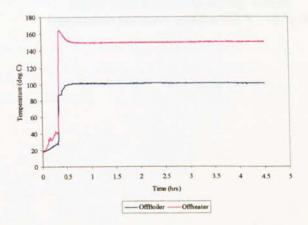
Figure B.42 Airless drying: boiler and off-heater temperature profiles  $(T_{ss} = 150 \text{ °C})$
