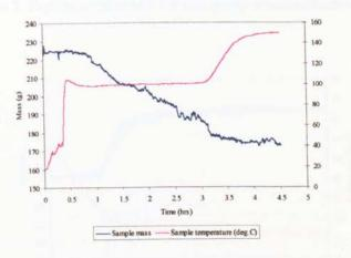
Figure B.41 Airless drying: sample temperature and mass profiles  $(T_{ss} = 150 \text{ °C})$
