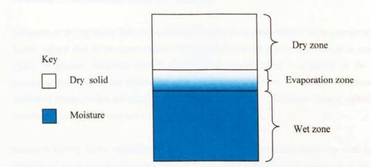
Figure 5.6 Moving boundary (receding front) drying mechanism
