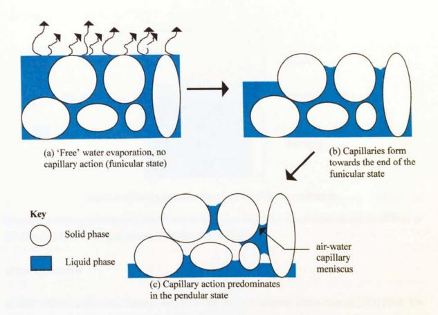
Figure 5.4 Schematic of porous solid containing interconnecting pores and channels.
