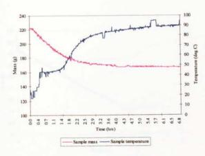
Figure B.30 Air drying of electro-porcelain  $(T_a = 90 \text{ °C}, \text{ no humidity control})$
