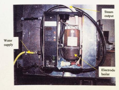
Figure 6.8 Direct steam injection humidifier (convective air dryer)
