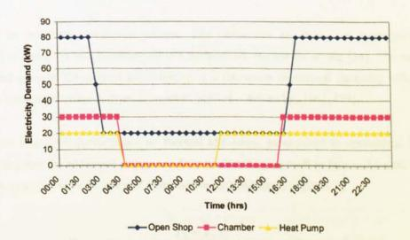
Figure 8.6 A comparison between shop, chamber and heat pump drying profiles
