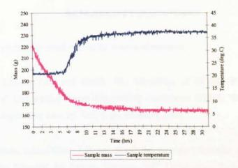
Figure B.43 Heat pump drying: sample temperature and mass profiles (40 °C, 18 % rh)
