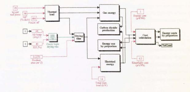
Figure 7.2 Simulink model (convective air drying)
