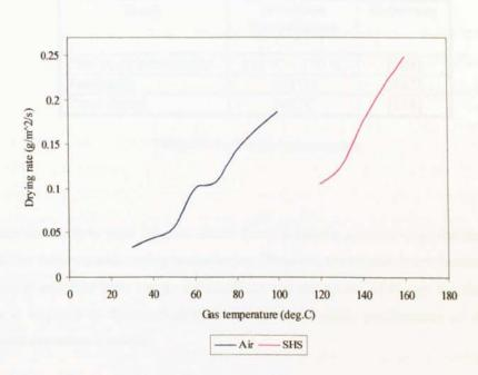
Figure 6.53 Drying rate comparison: air drying vs. airless drying
