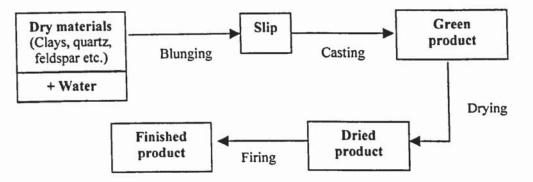
Figure 8.0 Sanitaryware production process
