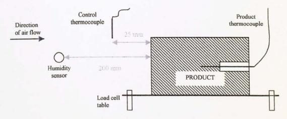
Figure 6.7 Humidity and thermocouple sensor locations
