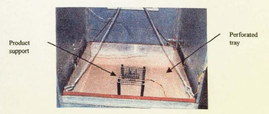
Figure 6.42 Heat pump tray and sample support
