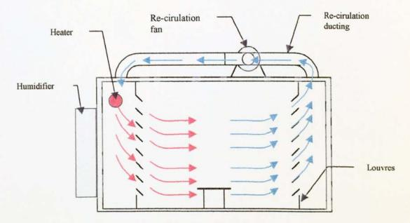
Figure 6.5 Air dryer cross-section
