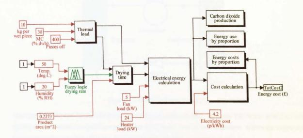
The Simulink model for heat pump dehumidification drying is given in figure 7.7.
