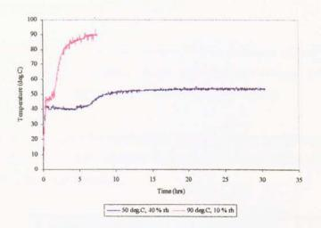
Figure 6.11 Convective air drying profile (product temperature)
