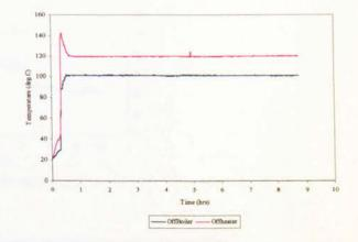
Figure B.35 Airless drying: sample temperature and mass profiles ( $T_{ss} = 120$  °C)
