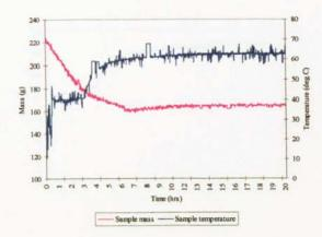
Figure B.17 Air drying of electro-porcelain ( $T_a = 60 \text{ °C}, 20 \text{ \% rh}$ )
