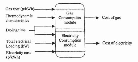
Figure 7.4 Energy calculation by fuel type
