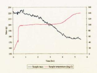
Figure B.39 Airless drying: sample temperature and mass profiles ( $T_{ss} = 140 \text{ °C}$ )
