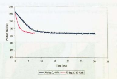
Figure 6.10 Convective air drying profile (product weight loss)
