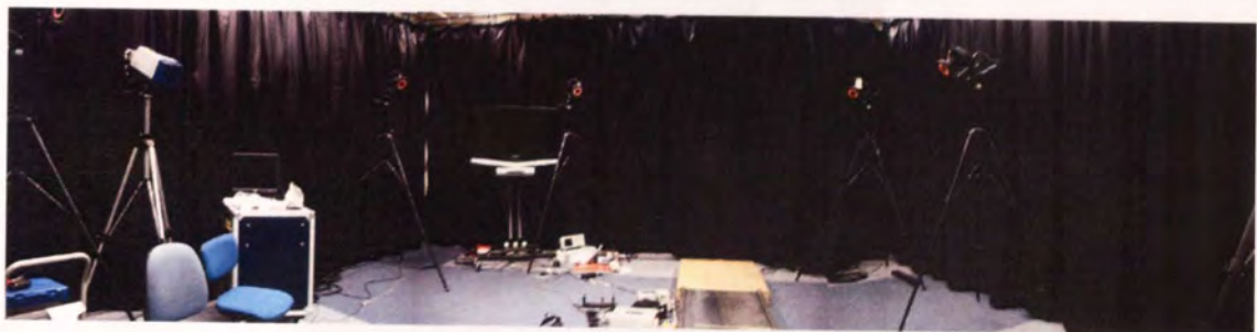
Figure A.5: Panoramic view of the experimental area, with the sensing plate and motion capture system.
