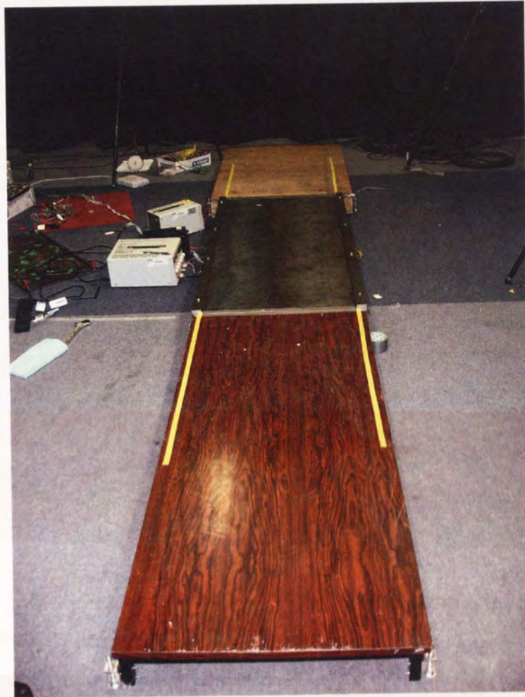
Figure A.3: The full walkway with the gait initiation platform, sensing platform and gait termination platform respectively.
