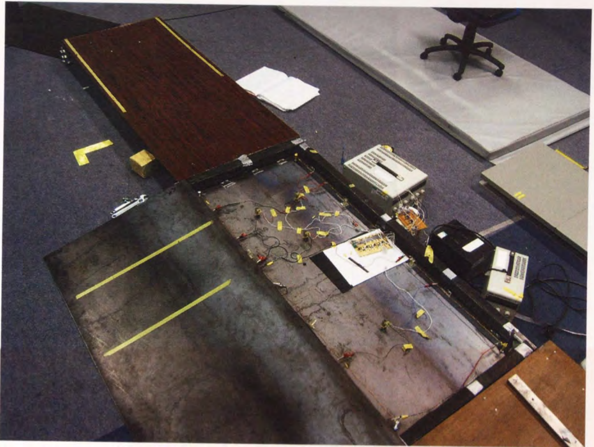
Figure A.4: The sensing platform with the top plate removed showing the baseplate containing the sensors and electronic signal conditioning circuits
