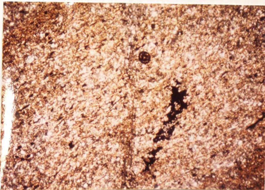
PLATE 6:5B SHEAR PLANE (SAMPLE S32/1/A) PERPENDICULAR TO BEDDING
