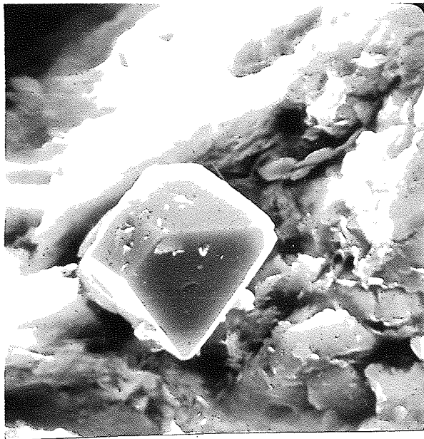
PLATE 6:14 AUTHIGENIC MAGNETITE BOREHOLE SAMPLE, DEPTH 11.7m
