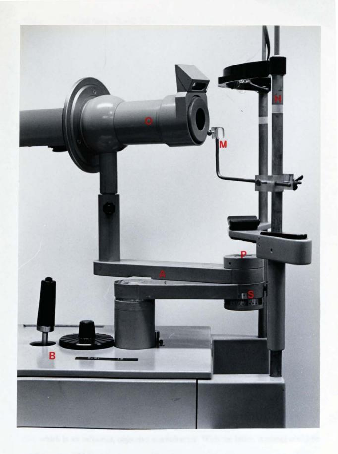
Fig. 3.3 Photograph of the modified arm built for the Hartinger coincidence optometer. Key: O -optometer; A -modified arm; P -point of rotation; B -moveable base; S -scale; H -headrest; M -mirror. See text.
