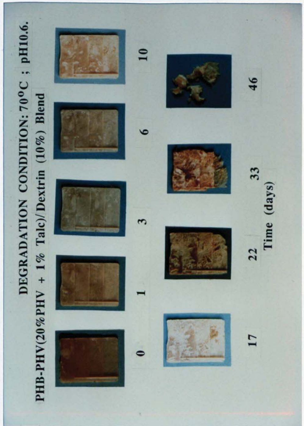
Plate 4.24 Injection moulded plaques: Photographic illustration of hydrolytic degradation.
