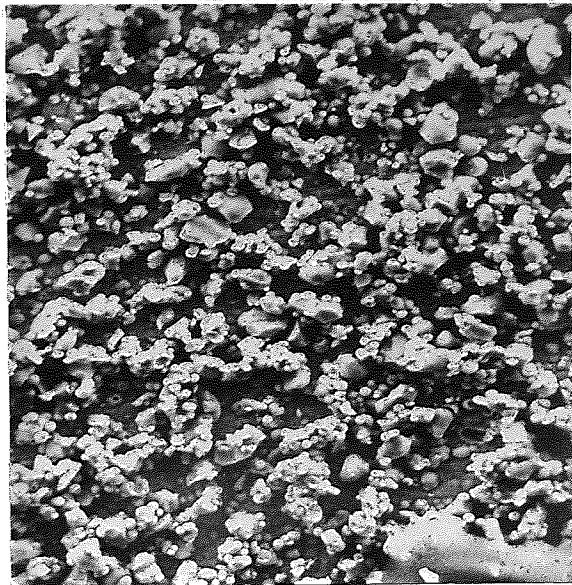
FIGURE 56 SURFACE OF NICKEL+CHROMIUM COMPOSITE DEPOSIT AFTER 12 HOURS PLATING (x 1000 SCANNING ELECTRON MICROGRAPH)
