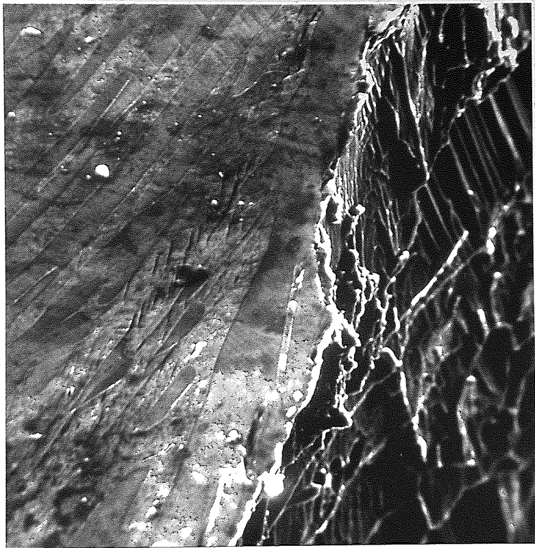
FIG. 68 (d) FRACTURE EDGE FROM SPECIMEN FORGED AT 950°C AND DOUBLE HEAT TREATED
