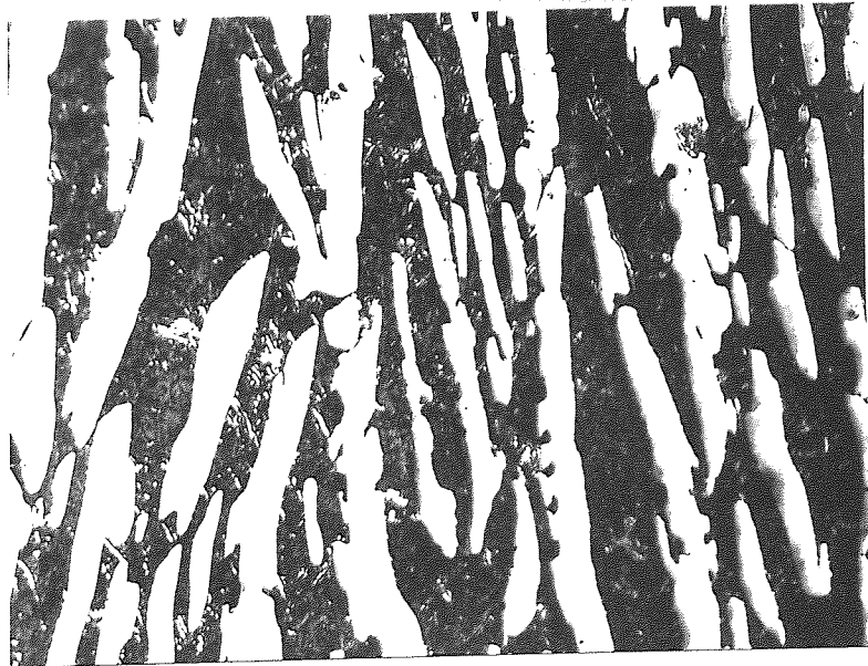
FIG. 60 (a) COOLED FROM 1080^{\circ}\text{C} TO 970^{\circ}\text{C} S.T.A. 900^{\circ}\text{C}/500^{\circ}\text{C} (b) COOLED FROM 1080^{\circ}\text{C} TO 880^{\circ}\text{C} S.T.A. 900^{\circ}\text{C}/500^{\circ}\text{C} x 800 (c) COOLED FROM 1080^{\circ}\text{C} TO 770^{\circ}\text{C} S.T.A. 900^{\circ}\text{C}/500^{\circ}\text{C} Ti/6Al/4V
