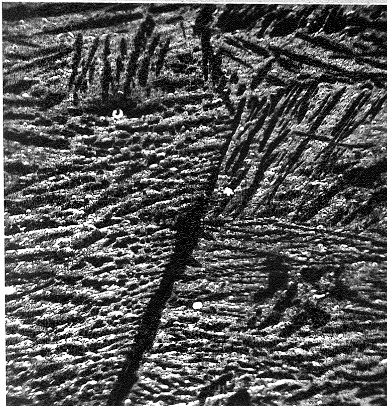
FIG. 61 (a) CRACK TIP OF DOUBLE HEAT TREATED IMI 700 x 270
