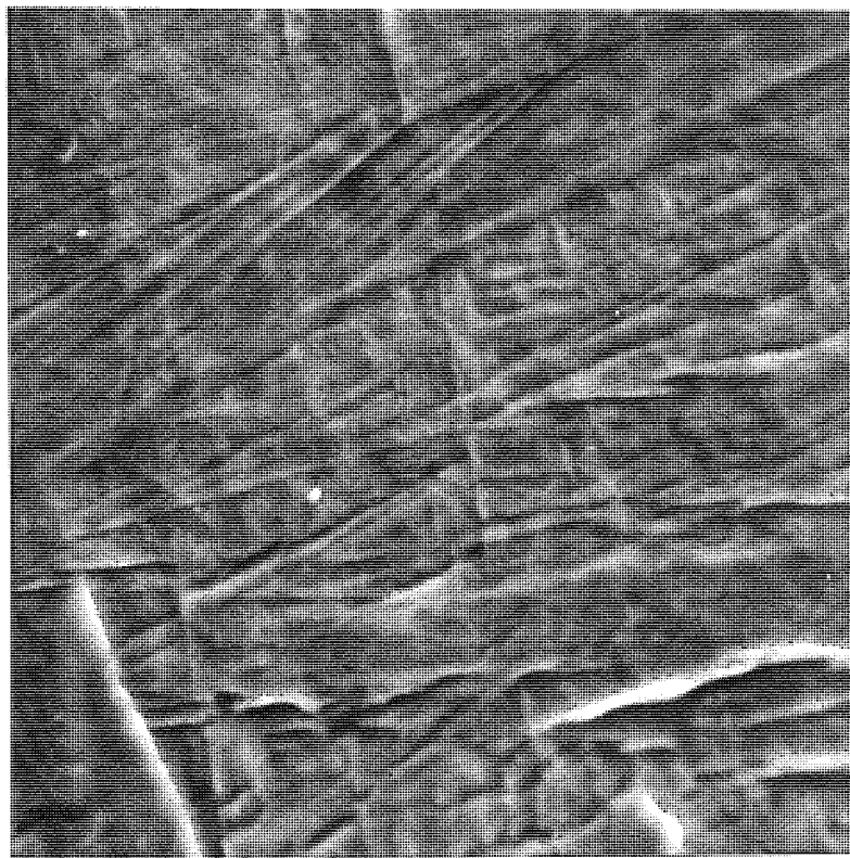
FIG. 56 (b) MICROGRAPH NEAR FRACTURE EDGE OF 1020°C SOLUTION TREATMENT - Ti/6Al/4V
