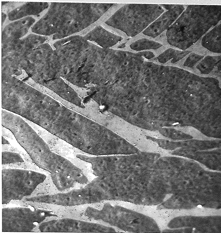
FIG. 65 (a) COOLED FROM 1020°C TO 650°C S.T.A. 800°C WQ/510°C
