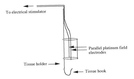
**Diagram 2.1** Representation of the tissue holder and field stimulators used with the guinea-pig ileal, right atrial and vas deferens preparations. Tissues were held between the field electrodes using cotton loops to the tissue hook (ileum and vas deferens) or by attachment to the tissue hook directly (left atrium).Cotton loops attached the tissues to a force transducer positioned above.
