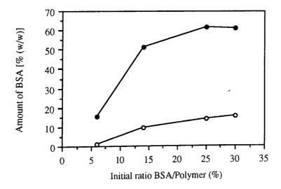
Figure 2.13 - Variation of the amount of BSA encapsulated with the initial ratio BSA/PLA (Mwt 2000 Da): (•) - percentage of BSA encapsulated. (o) - percentage of BSA in the final composition of the formulation.
