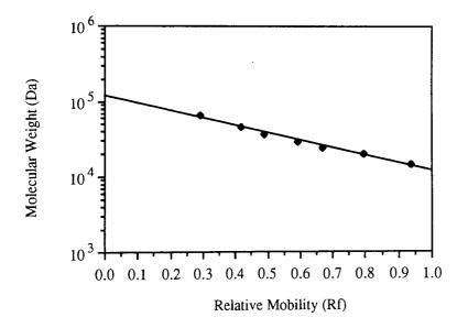
Figure 2.3 - Calibration curve (r = 0.993) for the estimation of the molecular weight of proteins by SDS-PAGE, using the molecular weight markers described in table 2.3.
