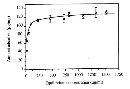
Figure 3.9 - Langmuir isotherm of BSA adsorption onto PLA (Mwt 2000 Da) microspheres (mean  $\pm$  sd; n = 3).
