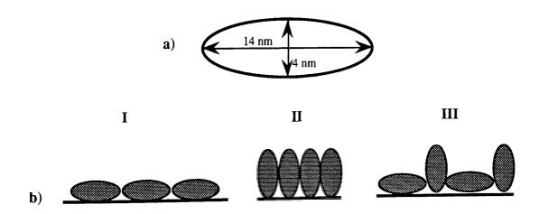
Figure 3.14 - a) Diagram of the ellipsoidal model of the BSA molecule with the approximate dimensions calculated by Squire *et al.* (1968). b) Adsorption of BSA: I) side-on; II) end-on; III) mixed process.
