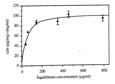
Figure 3.11 - Langmuir isotherm of  $\gamma$ -globulins adsorption onto PLA (Mwt 2000 Da) microspheres (mean  $\pm$  sd; n = 3).
