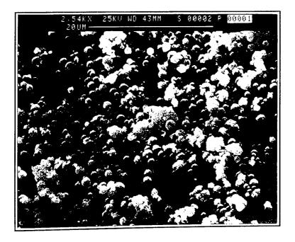
Figure 5.3 - Scanning electron micrograph of PLGA (50:50) microspheres containing 1.7% (w/w) of TT (mean size = 1.0  $\mu$ m,  $\sigma_g$  = 1.6; n = 306 particles).
