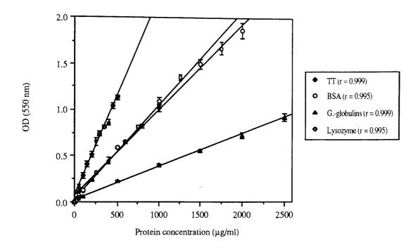
$\underline{Figure~2.1}$  - Calibration curve for the estimation of proteins by the standard protocol of the bicinchoninic acid protein assay.
