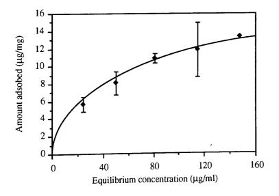
Figure 3.7 - Langmuir isotherm of TT adsorption onto PLA (Mwt 2000 Da) microspheres (mean  $\pm$  sd; n = 3).
