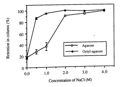
Figure 4.3 - Influence of the ionic strength of the eluent on the retention of PLA (Mwt 2000 Da) microspheres (n = 3; mean  $\pm$  sd).
