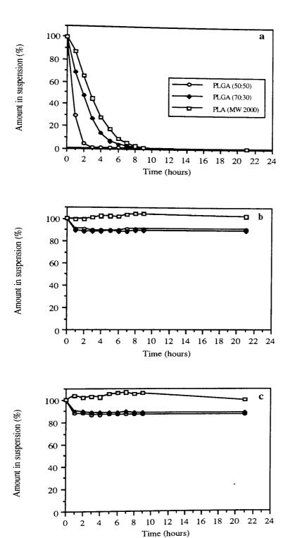
Figure 2.16 - Degradation of PLA/PLGA microspheres at different pH values: a) 0.1 M NaOH + 5% SDS, pH 11.7; b) PBS + 5% SDS, pH 7.4; c) 0.1 M HCl + 5% SDS, pH 1.0.
