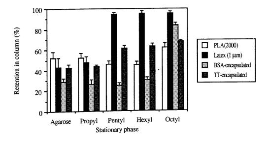
Figure 4.5 - Final retention by various stationary phases of the different proteinencapsulated formulations, compared with latex microspheres of a similar particle size (mean  $\pm$  sd; n = 3).
