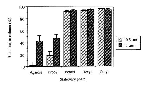
Figure 4.4 - Particle size dependence of the HIC method used in these studies as measured using two different sizes of polystyrene particles (n = 3; mean  $\pm$  sd).
