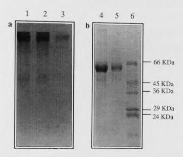
Figure 2:17 - SDS-PAGE (12% gels) of tetanus toxoid (a) and BSA (b). Lanes: 1) Tetanus Vaccine BP in Simple Solution; 2) TT before encapsulation in PLA (Mwt 2000 Da) microspheres; 3) TT after release from microspheres; 4) BSA before encapsulation in PLA (Mwt 2000) microspheres; 5) BSA after release from microspheres; 6) Molecular weight markers.
