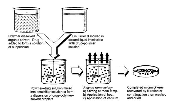
Figure 1.1 - Microsphere formation by emulsification/solvent evaporation (adapted from Watts et al., 1990).
