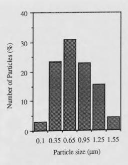
Figure 2.6 - Particle size distribution of PLA (Mwt 2000 Da) microspheres prepared by method D using a high speed homogeniser ( $\geq$  10000 rpm). Mean particle size = 0.7  $\mu$ m;  $\sigma_g$  = 1.8 (n = 231 particles).
