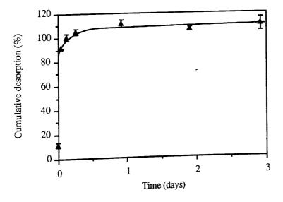
Figure 3.17 - Desorption profile of  $\gamma$ -globulins adsorbed onto PLA (Mwt 2000 Da) microspheres (in phosphate buffer 20 mM, pH 7.5; n = 3  $\pm$  sd).
