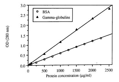
Figure 3.1 - Calibration curve for the estimation of BSA (r = 1.000) and  $\gamma$ -globulins (r = 0.999) by direct spectrophotometry.
