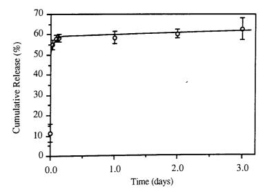
Figure 2.14 - Release of BSA from PLA (Mwt 2000 Da) microspheres in 20 mM phosphate buffer, pH 7.5. Vertical bars indicate the standard deviation at each point (n = 4).
