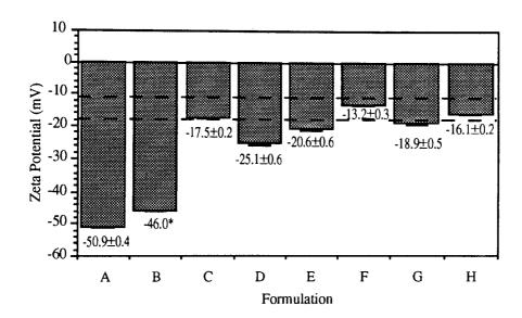
Figure 4.8 - Surface charge of the various formulations measured as zeta potential (mean  $\pm$  sd; n = 3). Legend: A) Latex microparticles (1  $\mu$ m); B) PLA microspheres prepared with Tween 80; C) PLA microspheres prepared with PVA; D) BSA-encapsulated PLA microspheres; E) BSA-adsorbed PLA microspheres; F) TT-encapsulated PLA microspheres; G) TT-adsorbed PLA microspheres; H)  $\gamma$ -globulins-adsorbed PLA microspheres. (\* n = 2).
