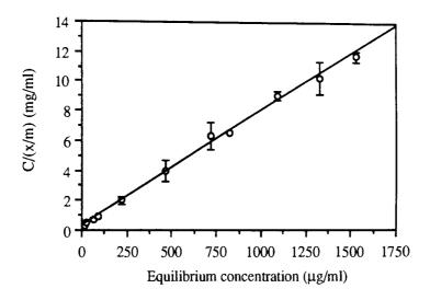
Figure 3.10 - Langmuir plot (r = 0.998) corresponding to the BSA adsorption isotherm of fig. 3.9 (mean  $\pm$  sd; n = 3).
