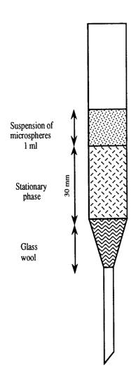
Figure 4.1 - Diagram of a HIC column prepared using a glass Pasteur pipette as described in the text.
