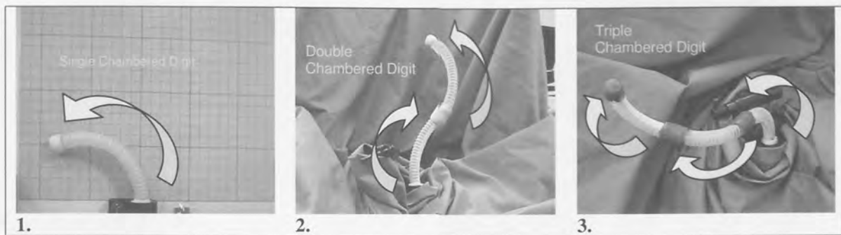
Figure 4.12 Flexible digits with one, two and three chambers
