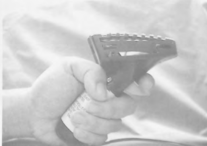
Figure 6. 7 A resistive trigger input device
