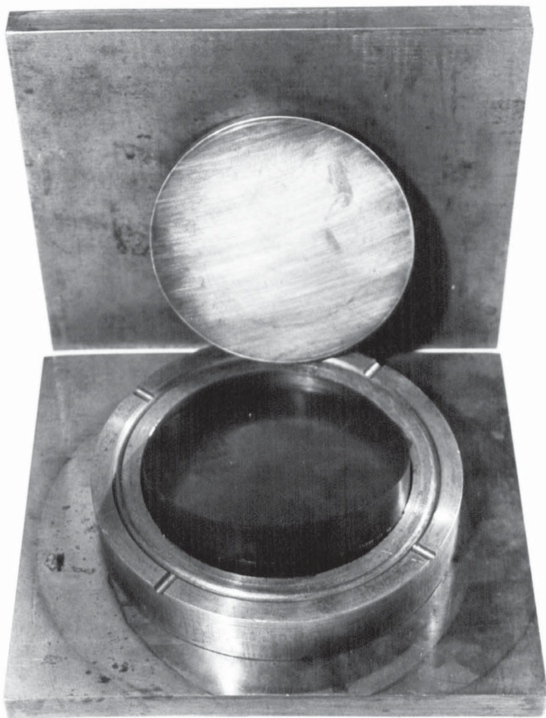
Plate 7 Typical elastomer layer mould.
