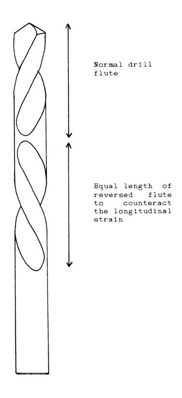
Figure 90 - Drill Modification Design
