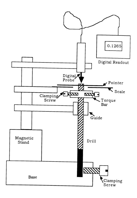
Figure 89 - Drill Extension Testing Machine
