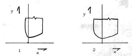
These wheels only produce the predicted flute shape over the cutting edge. The profile of the secondary or trailing half is uncontrolled.
