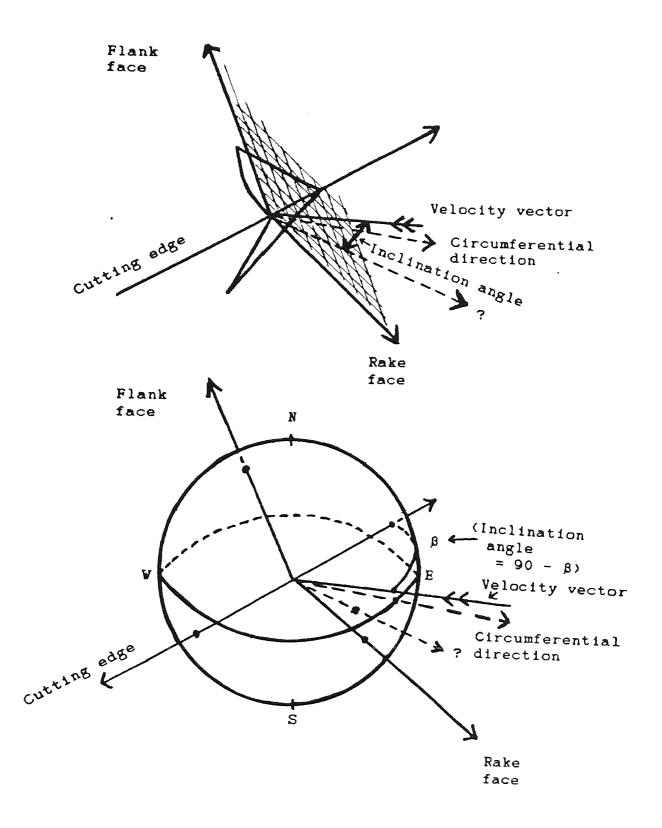
Figure 28 - Spherical Representation
