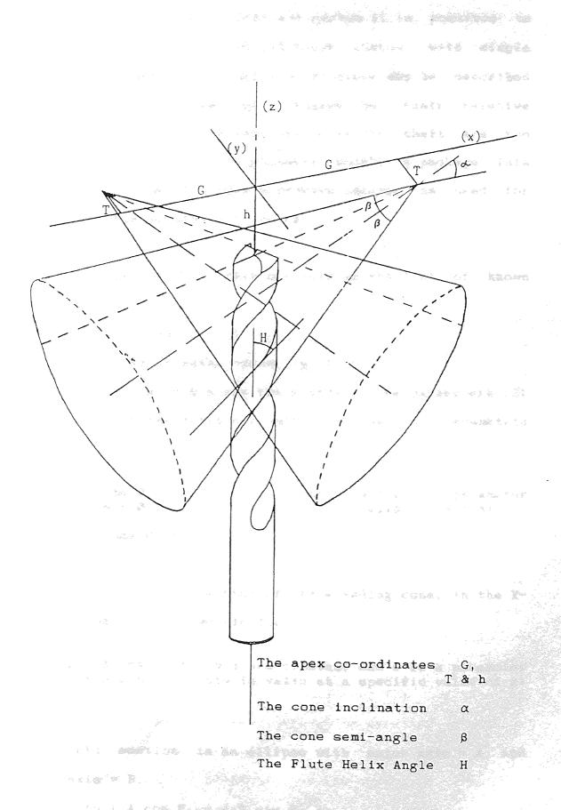
Figure 13 - Grinding Cones and Drill Parameters
