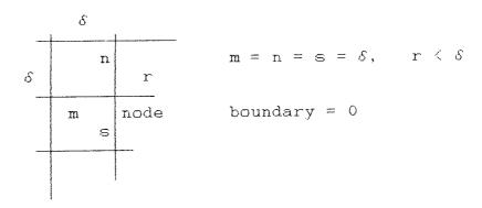
As this alteration is only valid at the boundary and for the examination of torsion the boundary value is fixed at zero, this is a simple adjustment to the spreadsheet equation, i.e., it only requires adjustment to the value of the denominator. This is normally = 4 and will be increased by the change.
