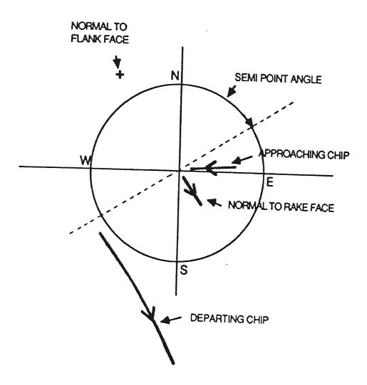
Figure 3.1 Stereographic Representation of the Cutting Action of a Straight Edge Twist Drill [14]
