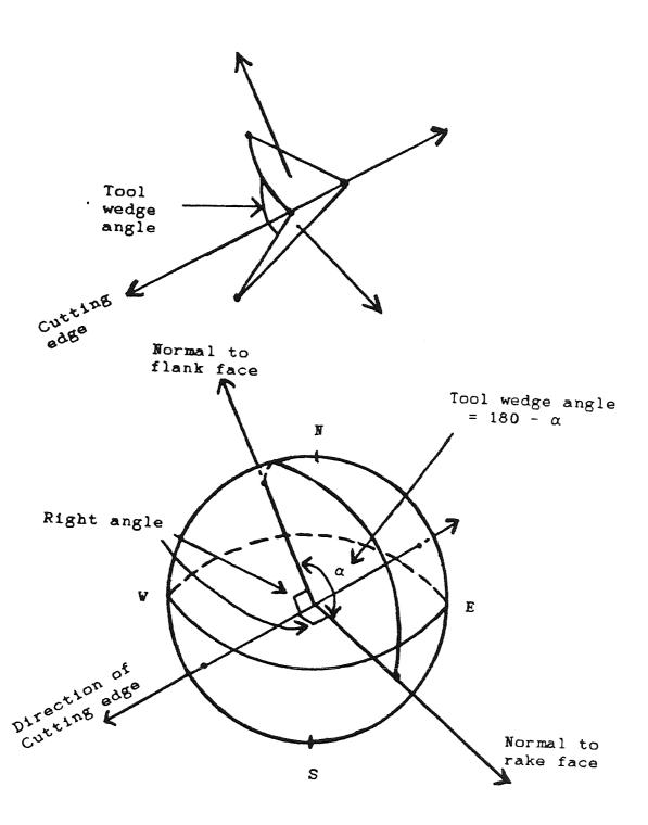
Figure 26 - Spherical Representation of Tool Wedge Angle
