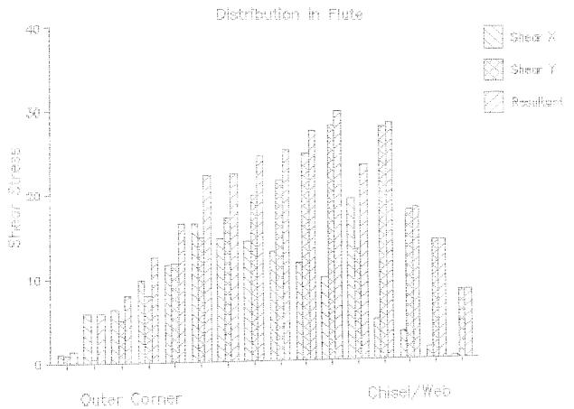
Shear stress in terms of the slope of the numerical distribution of stress function
