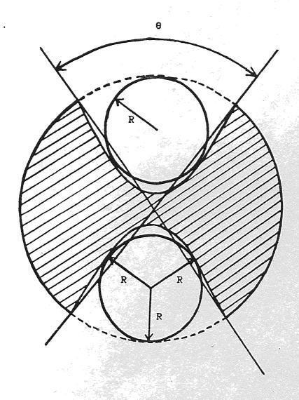
Figure 23 - Optimisation of Drill Stiffness
