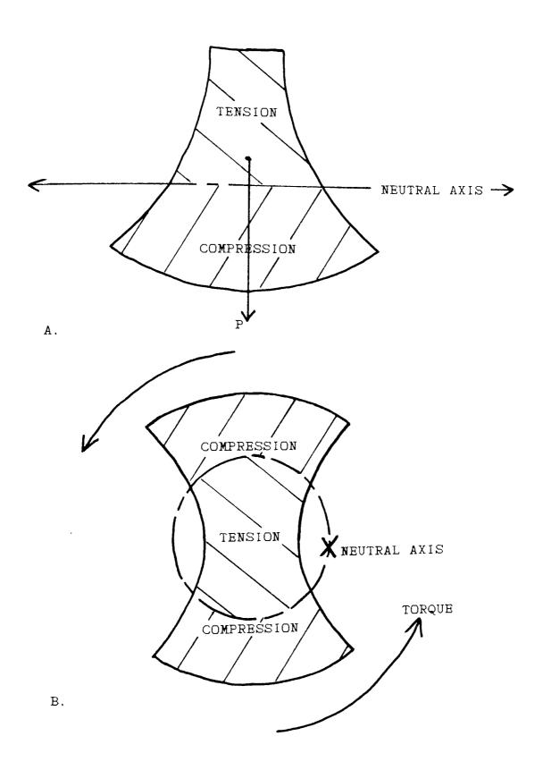
Figure 78 - Bending Model Strain Distribution & Cross Section of Drill under the Influence of Torsion
