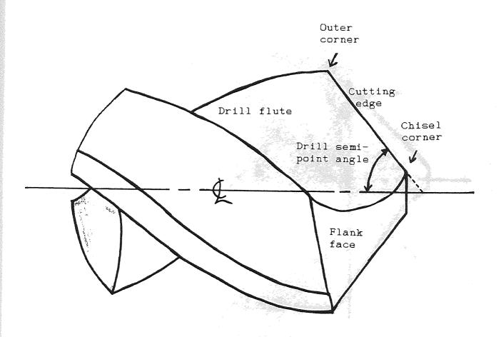
Figure 19 - Side Elevation Normal to Cutting Edge
