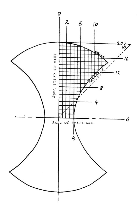
Figure 70 - Cross Section showing the Drill Mesh used for the evaluation of Finite Difference Equations
