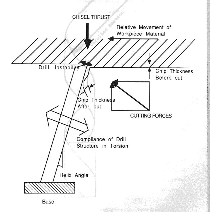
Figure 68 - Dynamic drilling Model
