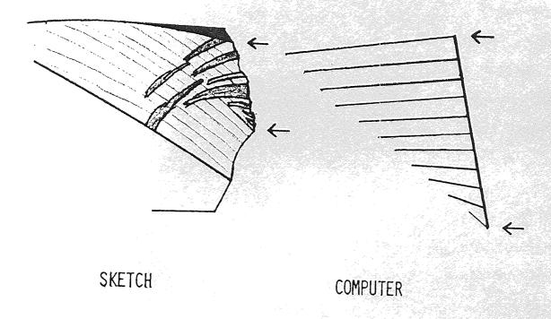
Figure 64 - Sketch vs Simple Computer Representation of Chip Flow [14]
