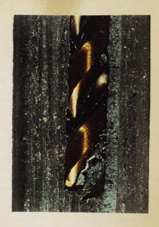
Figure 87 - Photograph of Broken Drill in Test Block
