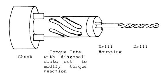
Figure 91 - Drill Mounting Design
