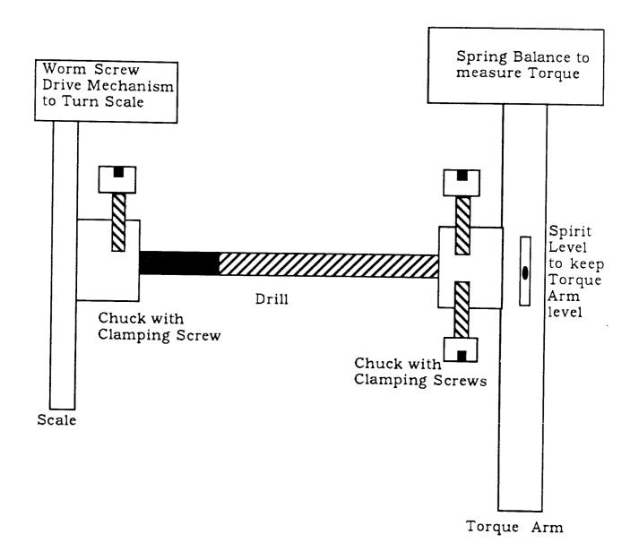
Figure 88 - Drill Torque Testing Machine
