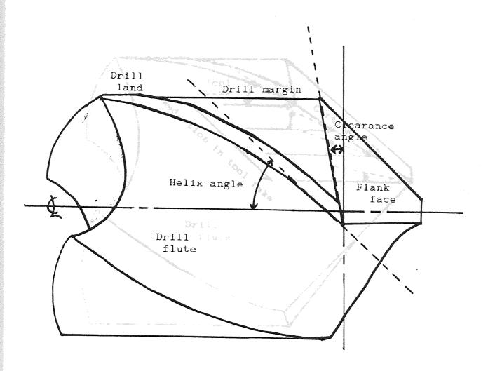
Figure 20 - Side Elevation of Outer Corner
