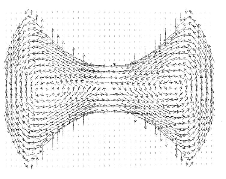
Figure 72 - Turbo Pascal Display of Torsional Shear Stress Distribution
