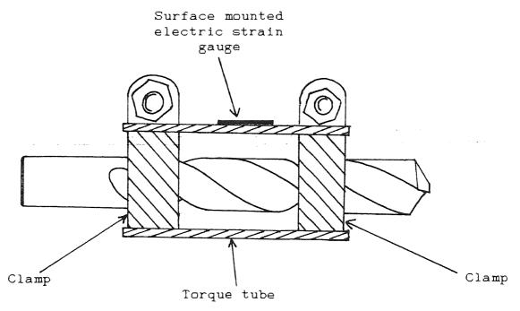
Figure 11. - Schaterin's Torque Tube
