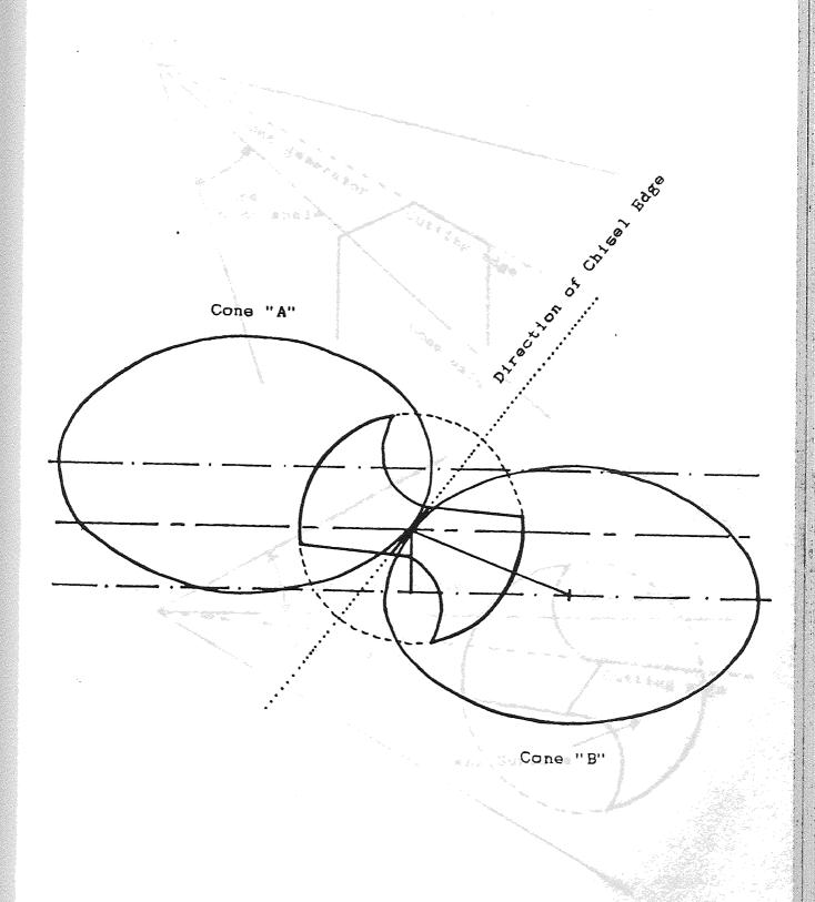
Figure 17 - Intersection of the Ellipses at the Tool Tip
