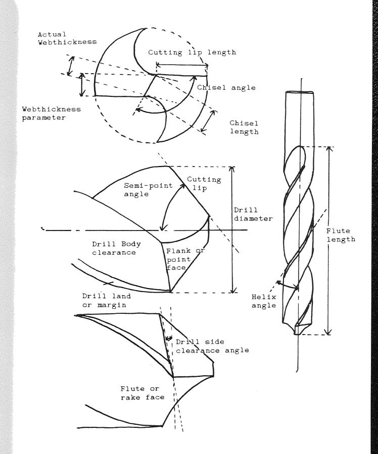
Figure 7 - Geometric Reference Values of Drill Form
