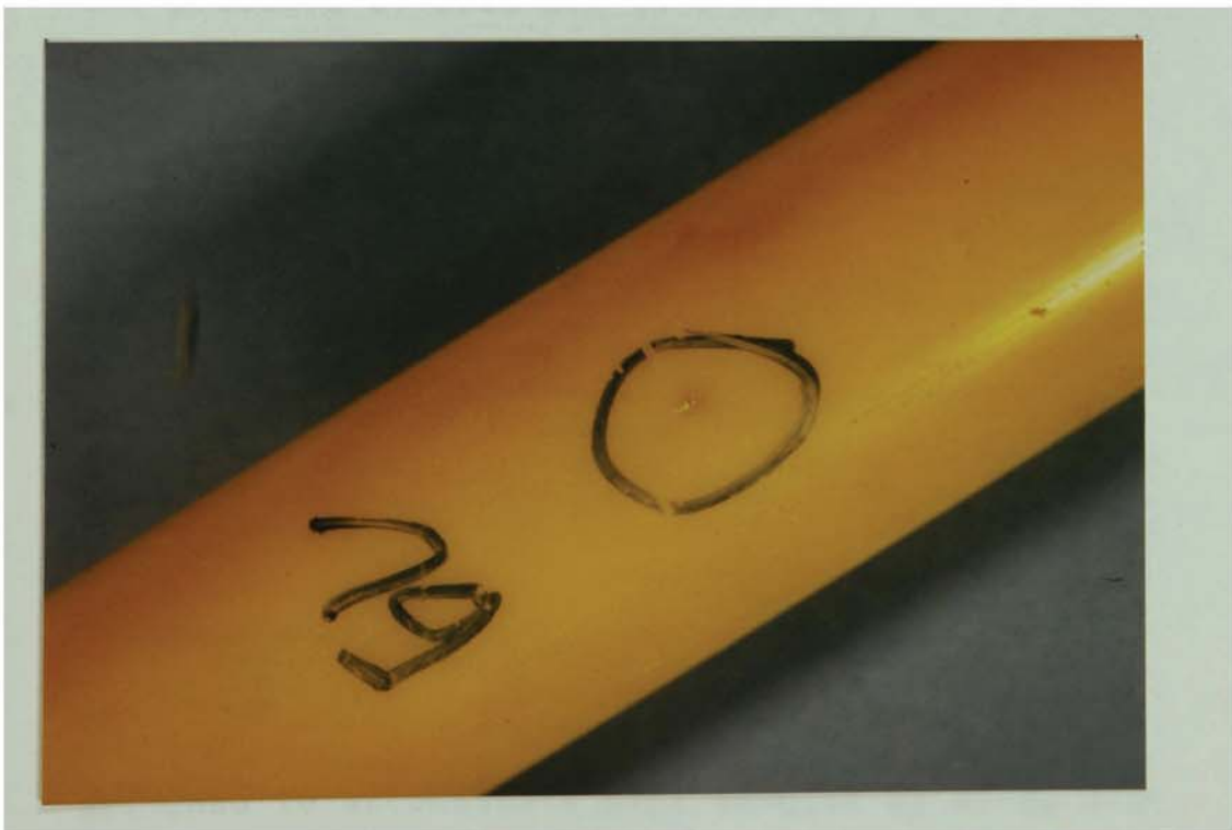
Fig. 5.4 Photograph of Typical Brittle Failure Point
