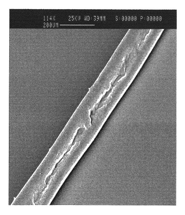
Figure 3.12 SEM of 10% PCL fibre after 500% extension.
