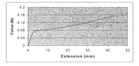
**Figure 3.16** Force-extension curve of a 10% w/v fibre hot drawn at 37°C to 200% extension and tested once cooled at room temperature
