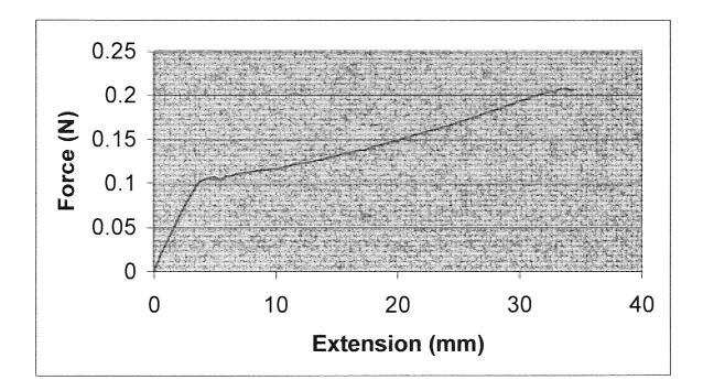
**Figure 3.17** Force-extension curve of a 10% w/v fibre hot drawn at 37°C to 500% extension and tested once cooled at room temperature
