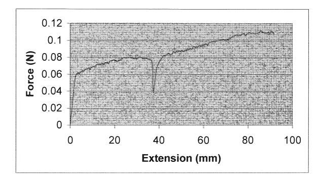
Figure 3.14 Force-extension curve of a 10% w/v fibre cold drawn to 500% extension.
