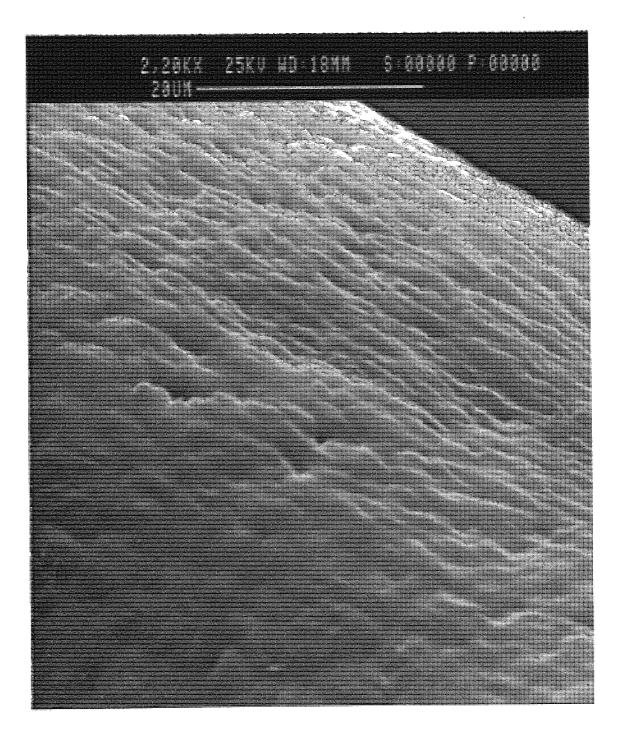
Figure 3.6 SEM of the surface topography of as-spun PCL fibre produced from a 10% w/v polymer solution
