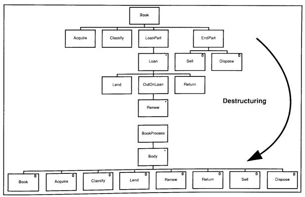
Figure 5.8. Destructuring of process structures.
