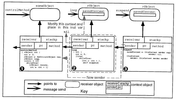
Figure 4.9. Suspend mechanism.
