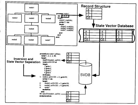
Figure 6.1. The separation and storage of state vectors.
