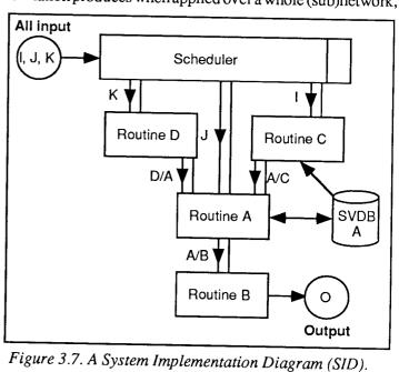
vector separation and inversion, to implement an entire specification on a single machine if desired. A more detailed explanation of state vector separation can be found in Chapter 6.
