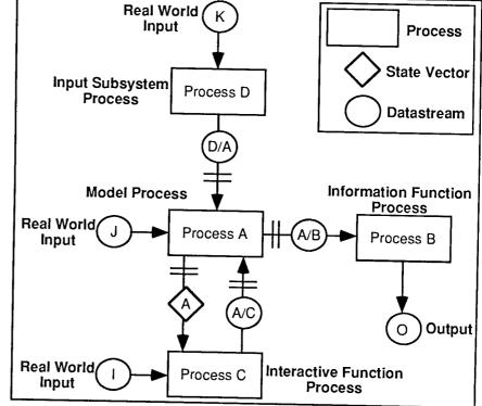
Figure 3.3. A System Specification Diagram (SSD).
