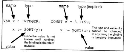
Figure 2.5. Binding mechanism in Pascal.
