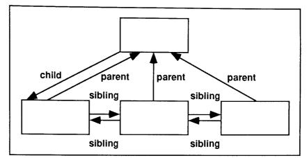
Figure 6.5. Node linkage in the representation of structure diagrams.
