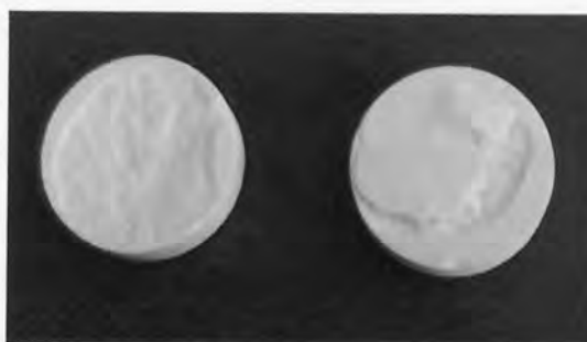
Figure 7.4: Capping and lamination on gum Arabic matrix tablets of cimetidine
