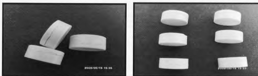
Figure 7.3: Tablet defect seen on binary composite matrices of grewia/ethyl cellulose (1:1 and 1:2)
